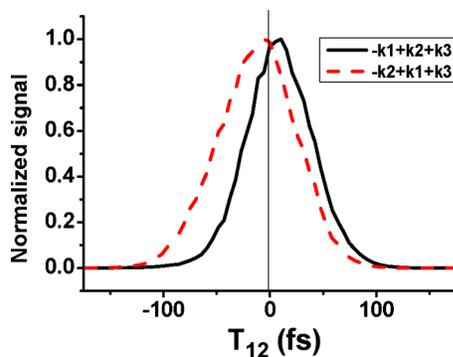
FIG. 7. Nonresonant signal from pure ethanol in two phase-matched directions ( $T_{23}=0$ ).
