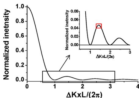
FIG. 10. Normalized intensity of nonlinear signal as a function  $\Delta k L / 2\pi$  given by Eq. (5). Inset: the range of possible values of  $\Delta k \times L$  given by our experimental conditions is marked by a small red square.
