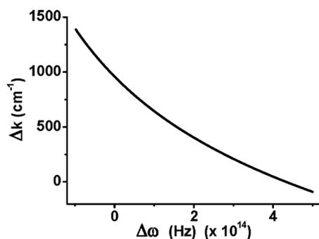
FIG. 9. The phase mismatch ( $\Delta k$ ) as a function of  $\Delta\omega$  in the triangular geometry ( $\gamma=3.1^\circ$  and  $\lambda=287$  nm).
