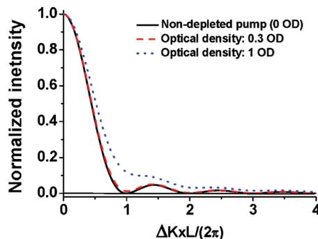
FIG. 11. Normalized intensity of nonlinear signal as a function  $\Delta kL/2\pi$  for the case of 0.3 OD (real condition, dashed red line), 0 OD (nondepleted pump, solid black line), and 1 OD (dotted blue line).
