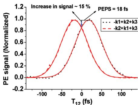
FIG. 2. An example of the PE signals detected in two phase-matched directions at  $T_{23}=1$  ps. The PEPS value is measured to be 18 fs. The maximum of signal is about 15% higher than the signal value at  $T_{12}=0$ .
