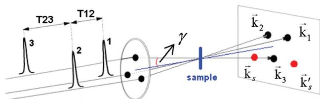
FIG. 1. Triangular geometry of the input beams in the PE setup. The PE signals are detected in two phase-matched directions,  $\vec{k}_s = -\vec{k}_1 + \vec{k}_2 + \vec{k}_3$  and  $\vec{k}'_s = -\vec{k}_2 + \vec{k}_1 + \vec{k}_3$ .
