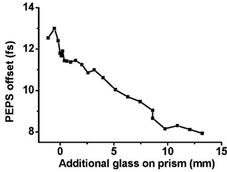
FIG. 6. An example of dependence of the PEPS offset on the chirp, obtained by increasing the length of glass in the compression stage prism through which the beam passes. The measurements were done on DPA in ethanol. ( $T_{23}=1$  ps).
