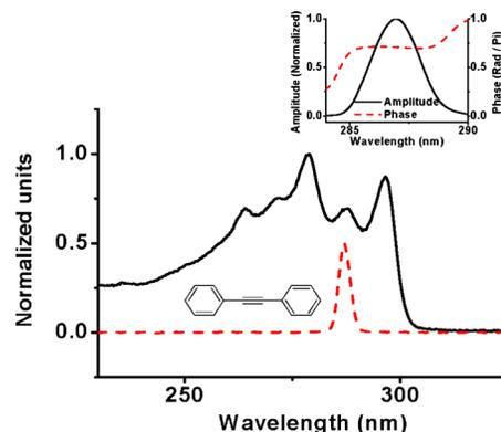
FIG. 3. Absorption spectrum of DPA (see scheme of the molecular structure) in ethanol (solid black line) and the excitation pulse spectrum (dashed red line). Inset: spectral amplitude and phase of the UV pulses at the sample position.
