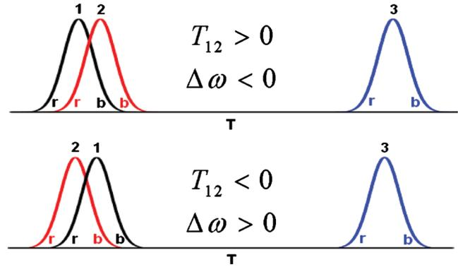
FIG. 8. Interaction of chirped pulses in the PE setup. In this scheme, pulses are positively chirped. "r" refers red chirp and "b" refers to blue chirp of the pulses.  $\Delta\omega$  is the average detuning of the interacting components of the first and second pulses from  $\omega_0$  defined by Eq. (2).
