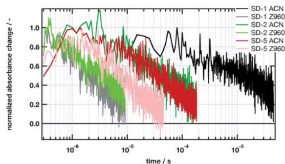
**Fig. 7** Transient absorbance decay of the oxidized state of **SD-1**, **SD-2** and **SD-5** sensitizers adsorbed on nanocrystalline TiO<sub>2</sub> films. The kinetics observed with acetonitrile, no iodide added (ACN) and in the presence of redox electrolyte Z960 under similar conditions.
