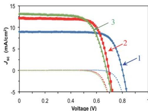
**Fig. 4** Current density–voltage curve under full sunlight (AM1.5G,  $100 \text{ mW cm}^{-2}$ ) and in the dark of devices sensitized with **SD-1** (blue, curve 1), **SD-2** (red, curve 2) and **SD-5** (green, curve 3) using a volatile electrolyte Z960.
