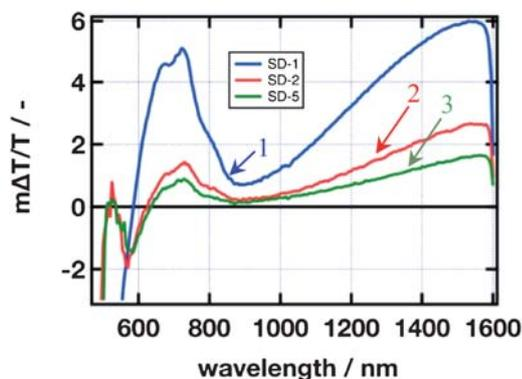
**Fig. 6** Photoinduced absorbance spectra of the TiO<sub>2</sub> photoanodes sensitized with three dyes of **SD-1** (blue, curve 1), **SD-2** (red, curve 2) and **SD-5** (green, curve 3),  $\lambda_{ex} = 470$  nm, repetition rate being 9 Hz.
