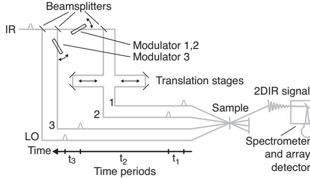
Fig. 2. A schematic drawing of the box-CARS 2D IR setup. An IR pulse is split into four pulses  $E_1$ ,  $E_2$ ,  $E_3$  and  $E_{LO}$ . Pulses 1 and 2 are transmitted together through one modulator before they are split, while pulse 3 is modulated independently. The three incident pulses generate the signal field  $E_{2DIR}$ , which is heterodyned with the local oscillator by spectral interferometry. The timing notation is defined at the bottom of the figure.
