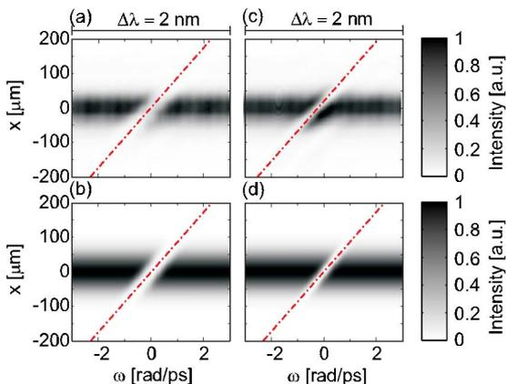
Fig. 1. (Color online) Space-frequency intensity distribution for the transmission of a single pixel set to zero—(a) experiment and (b) simulation—and for a  $\pi$  phase jump between two neighboring pixels—(c) experiment and (d) simulation. The dashed-dotted lines correspond to space-time coupling as predicted by Eq. (2).
