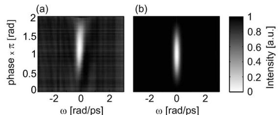
Fig. 2. (a) Measured and (b) simulated on-axis spectra ( $x = 0$ ) at the focal plane as a function of the phase step amplitude.
