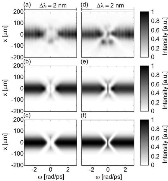
Fig. 3. Space-frequency intensity distribution for the double-pass configuration. Left column, transmission of a single pixel set to zero. Right column,  $\pi$  phase step. (a), (d) Experiments. Simulations (b), (e) with and (c), (f) without a second-order spatial phase.
