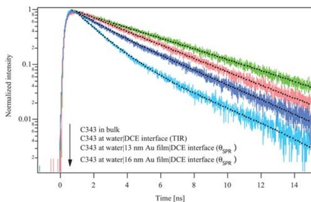
**Fig. 4** Fluorescence decay profiles, from top to bottom, of 30  $\mu\text{M}$  of Coumarin 343 in bulk water, at water|DCE interface under TIR condition and at water|Au film (16 or 13 nm)|DCE interface at the resonance angle. The fitting curves are marked by dotted lines.
