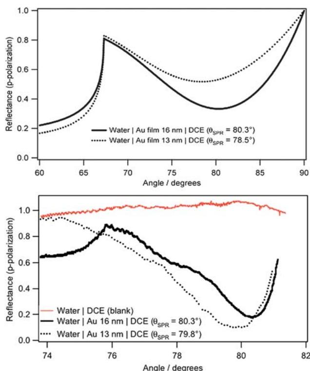
**Fig. 2** (Top) Calculated and (bottom) experimental SPR curves at water|DCE interface for an excitation wavelength of 544 nm (full line: 16 nm Au film, dotted line: 13 nm Au film).
