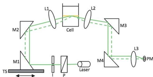
**Fig. 1** Schematic of the experimental setup of surface plasmon resonance at a liquid|liquid interface.
