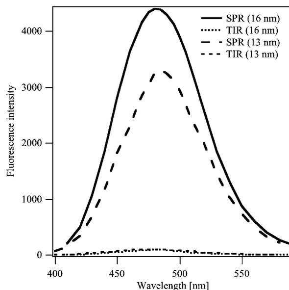
**Fig. 3** Emission spectra of the Coumarin 343 at water|Au film (16 nm or 13 nm)|DCE interface for TIR conditions and at the SPR. The excitation wavelength equals 450 nm.
