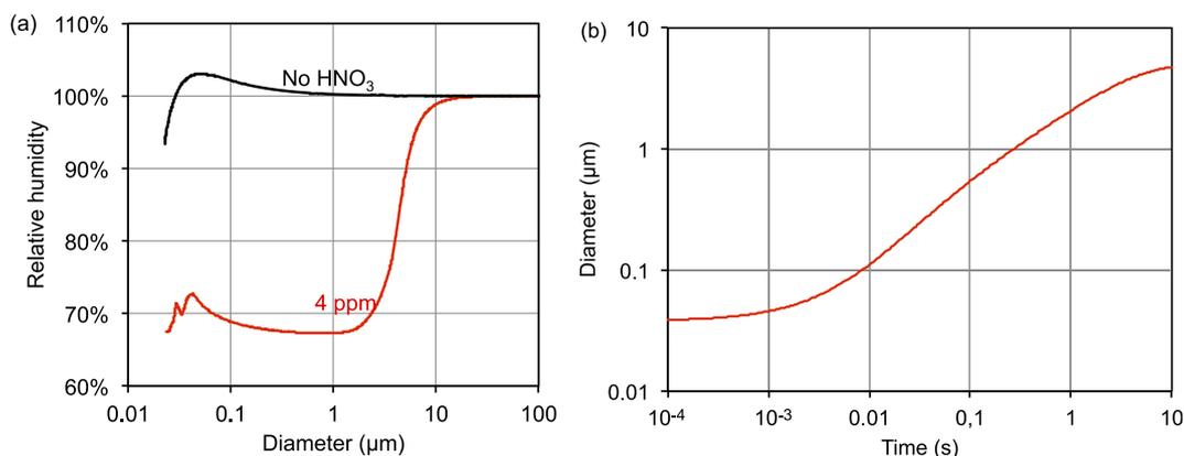
**Figure 8.** Laser-induced stabilization and growth of a cloud of 1000 particle  $\text{cm}^{-3}$ . (a) Köhler plot at 6 °C; (b) growth of ternary  $\text{HNO}_3\text{-H}_2\text{O-NH}_4\text{NO}_3$  particles at 2 °C, 90% RH and 4 ppm  $\text{HNO}_3$  (after [12]).
