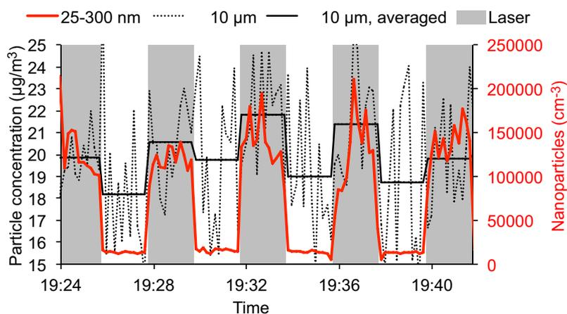
**Figure 6.** Quantitative observation of laser-induced condensation at 70% RH. The particle concentration is alternatively sampled close to the laser beam and under reference conditions. The difference between the measured concentrations is attributed to the effect of the laser.
