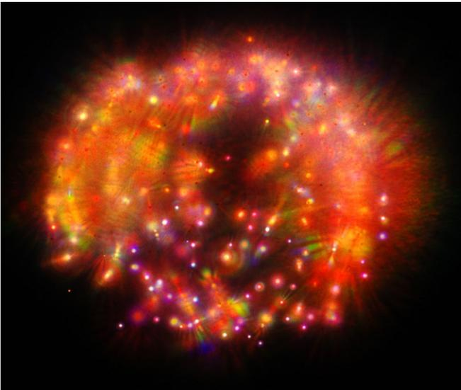
**Figure 3.** Multiple filamentation of a 3 J, 30 fs laser pulse of 10 cm diameter, imaged in real colour on a screen.
