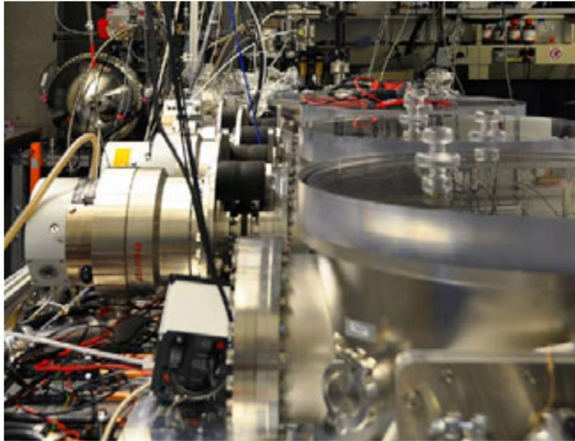
The attoliner (centre) enables ultrafast processes such as electron transfer in molecules to be studied at a higher temporal resolution.
