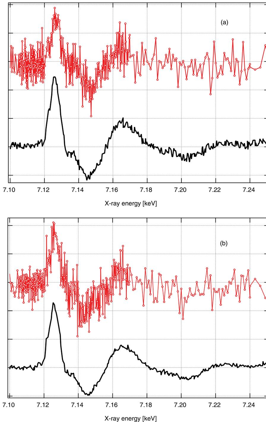
FIG. 7. (Color online) Representative single scans of the near-edge transient XAS of a 25 mM aqueous solution of  $[\text{Fe}(\text{bpy})_3]^{2+}$ , in transmission (a) and fluorescence (b) modes, collected using both the kHz (red circles) and high-repetition rate (black line) data acquisition techniques.
