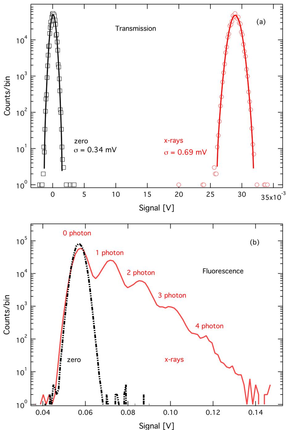
FIG. 5. (Color online) Pulse-height distribution of  $1 \times 10^6$  samples recorded in transmission mode (a) and fluorescence mode (b) at 7.125 keV for a 7 mM sample of  $[\text{Fe}(\text{bpy})_3]^{2+}$ . Gaussian fits to the histograms are shown as lines for the transmission signals. Note the clear peaks from multi-photon events in the fluorescence signal (0.56 photons/pulse).
