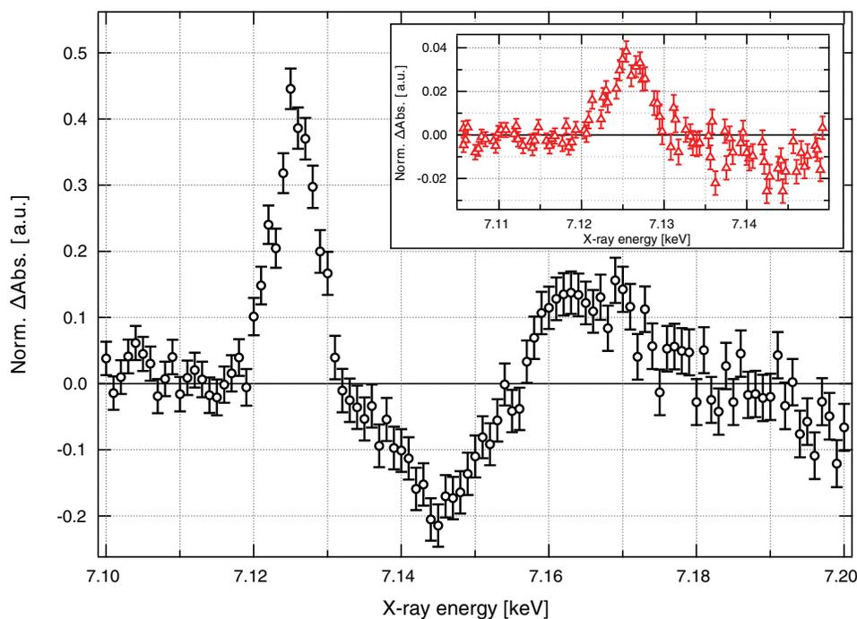
FIG. 8. (Color online) Average of 10 transient XAS scans 50 ps after excitation, of a 1 mM  $[\text{Fe}(\text{bpy})_3]^{2+}$  solution excited with a pump fluence of  $150 \text{ mJ}/\text{cm}^2$ . The inset shows a single transient XAS scan of a 25 mM aqueous solution of  $[\text{Fe}(\text{bpy})_3]^{2+}$  at 50 ps delay and collected in fluorescence yield mode with a pump fluence of  $13 \text{ mJ}/\text{cm}^2$ .
