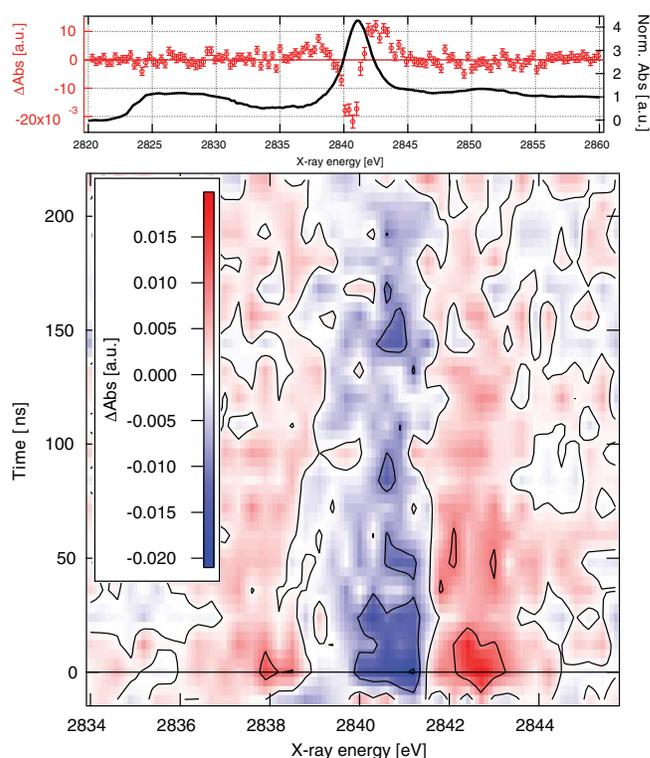
FIG. 9. (Color online) Top: Comparison between the ground-state XAS (black line) and transient XAS (red circles) measured 175 ps after time zero at the Ru  $L_3$  edge of an 80 mM solution of  $[\text{Ru}(\text{bpy})_3]^{2+}$  excited at 532 nm with a fluence of  $115 \text{ mJ/cm}^2$ . Note that the pre-edge signal on the ground-state XAS, from 2825 to 2830 eV, is the Cl K-edge absorption of the counter-ion. Bottom: Two-dimensional time-energy XAS measured under the same conditions.
