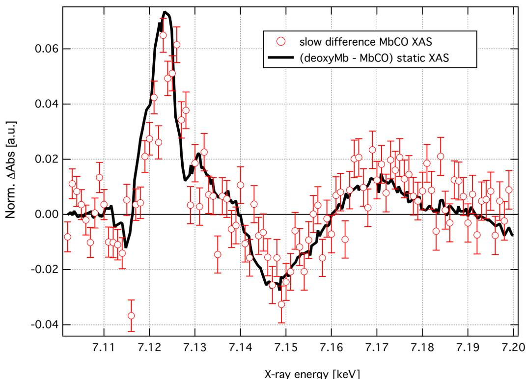
FIG. 12. (Color online) Transient XAS of 2 mM MbCO collected in fluorescence yield mode. The sample was excited at  $125 \text{ mJ/cm}^2$  laser fluence. The black curve represents the difference XAS based on the static spectra of deoxyMb and MbCO assuming an excitation yield of 21%.
