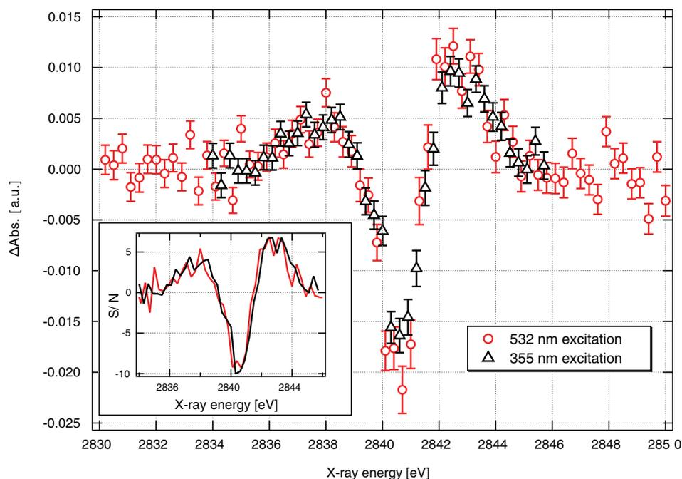
FIG. 10. (Color online) Comparison of the transient transmission XAS of an 80 mM aqueous solution of  $[\text{Ru}(\text{bpy})_3]^{2+}$  for excitation at 355 nm/ $\Delta t=5.6$  ns (black triangles) and 532 nm/ $\Delta t=175$  ps (red circles). The inset shows the S/N of the data with the 355 nm data being an average of 6 scans and the 532 nm data an average of 8 scans.
