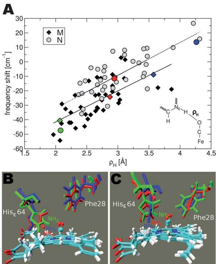
**Fig. 3** A: CO-stretch frequency shift distribution of all “dry” His<sub>ε</sub>64 M (diamonds) and N (circles) snapshots as a function of the His64-N<sub>ε</sub>H to CO oxygen distance  $\rho_H$ . The solid (M) and dashed (N) lines represent linear regressions. B: Representative His<sub>ε</sub>64 M structures selected from different regions of Figure A (color-coded) C: The same as in B but for His<sub>ε</sub>64 N.
