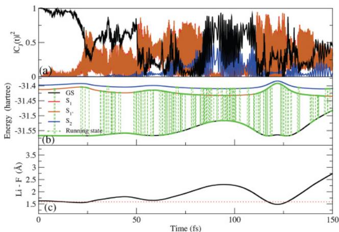
FIG. 6. (Color online) LiF under an isotropic pulse, with  $\omega = 0.005$  a.u. and  $A_0/c = 4.0$  a.u. For the description of panels (a)–(c) and the color coding, see Fig. 3.
